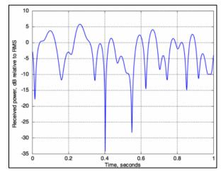
Figure F-9. Rayleigh Fading of a Signal Transmitted from a Moving Platform<sup>66</sup>
