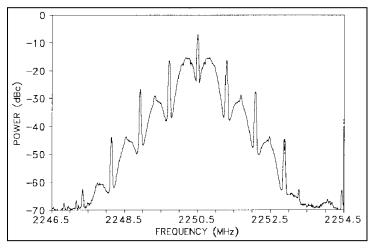
Figure A-6. Biø PCM/PM Signal
