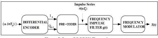
Figure 2-3. SOQPSK Transmitter
