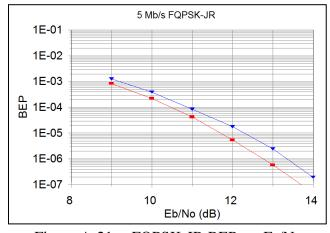
Figure A-21. FQPSK-JR BEP vs. E<sub>b</sub>/N<sub>0</sub>
