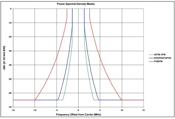
Figure A-29. Spectral Masks at -25 dBm
