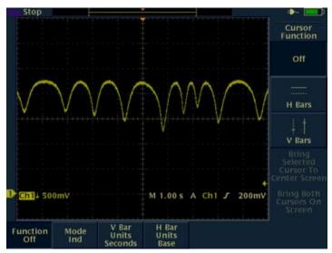
Figure F-10. S-band Telemetry Signal Received from an Aircraft in Flight<sup>67</sup>
