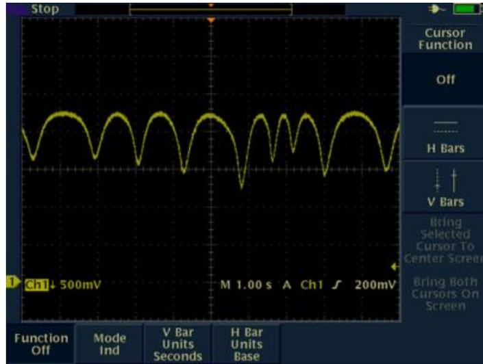
Figure F-10. S-band Telemetry Signal Received from an Aircraft in Flight<sup>67</sup>
