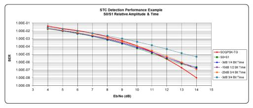
Figure E-4. Example Detection Curve Performance
