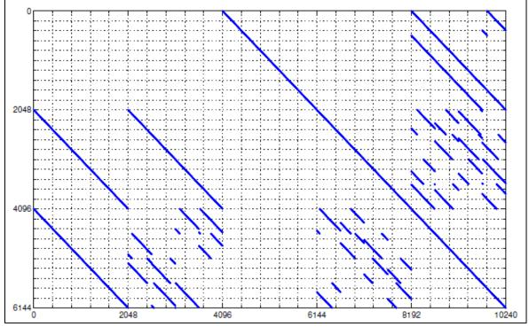
Figure D-2. Parity Check Matrix H for (n=8192, k=4096) Rate 1/2
