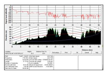
Figure F-13. EDX Signal Pro Path Loss Profile for the TX007 to RX007 Path
