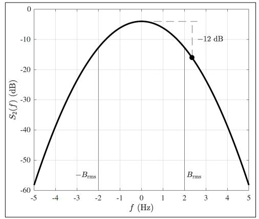
Figure H-1. The Gaussian Power Spectral Density  $S_2(f)$  given by Eq. 5 for  $B_{\rm rms}=2$  Hz
