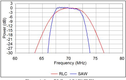
Figure A-9. RLC and SAW IF Filters
