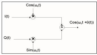
Figure A-14. OQPSK Modulator
