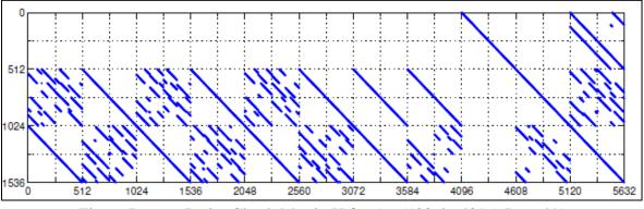
Figure D-6. Parity Check Matrix H for (n=5120, k=4096) Rate 4/5
