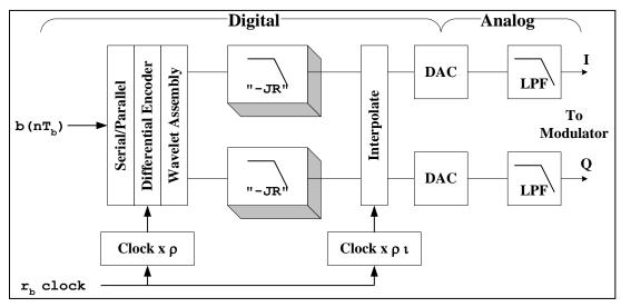
Figure 2-1. FQPSK-JR Baseband Signal Generator
