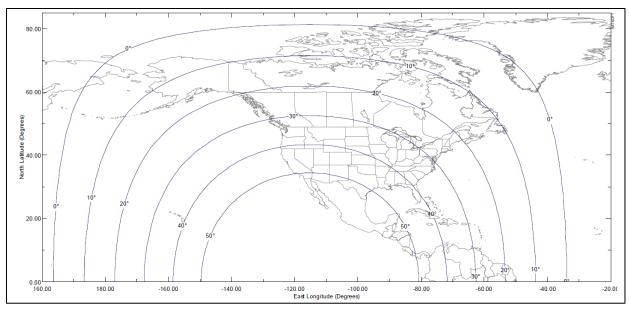
Figure F-4. Elevation Angles from Surface of the Earth to the 115.2° West Longitude Orbital Location
