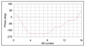
Figure A-22. Measured SOQPSK-TG Phase Trajectory
