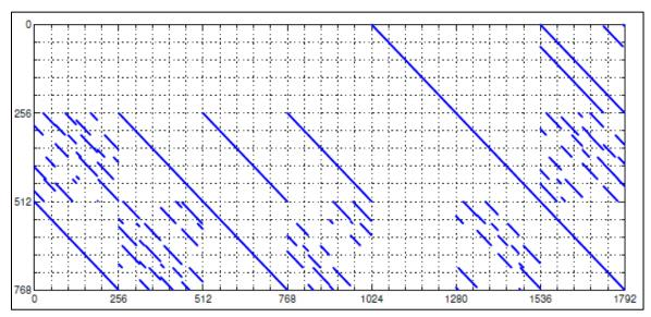
Figure D-3. Parity Check Matrix H for (n=1536, k=1024) Rate 2/3
