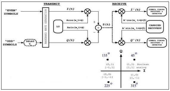
Figure B-2. OQPSK 106 Symbol-to-Phase Mapping Convention
