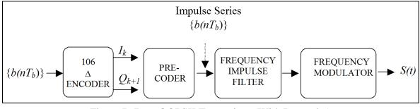
Figure B-7. OQPSK Transmitter (With Precorder)
