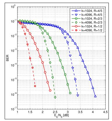
Figure D-10. LDPC Detection Performance with 4-state Trellis Demodulator
