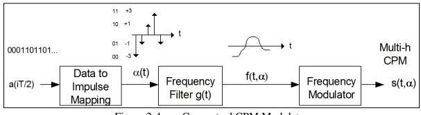
Figure 2-4. Conceptual CPM Modulator
