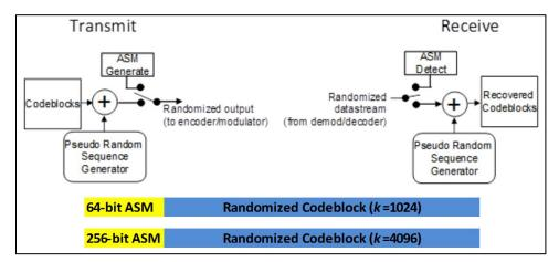
Figure D-8. ASM/Codeblock Structure
