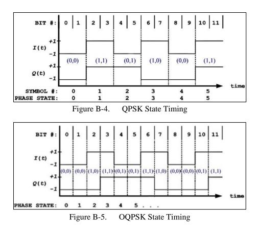
The Q channel half-symbol delay causes OQPSK phase trajectories to evolve on a halfsymbol (bit) rate basis. For the particular cases of FQPSK and SOQPSK-TG, carrier phase either remains unchanged or changes by  $\pm \pi/4$  or  $\pm \pi/2$  radians over the pending bit interval.
