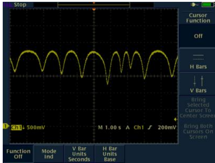
Figure F-10. S-band Telemetry Signal Received from an Aircraft in Flight 67
