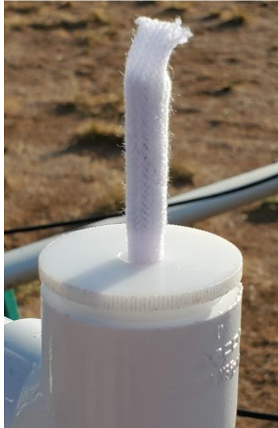
Figure 9. Desired Position of PT-1000 Temperature Probe and Wick
