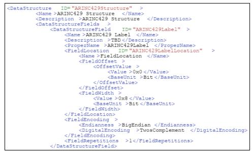
Figure 3-11. MDL Example Description of an ARINC 429 Data Structure
