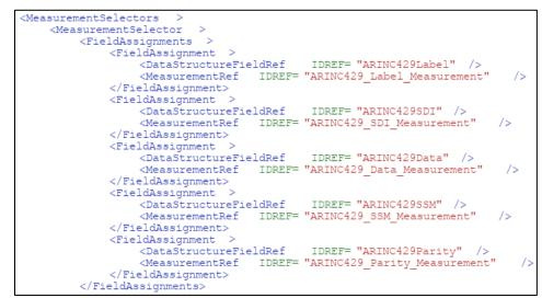
Figure 3-16. MDL Example Description of a Measurement Selector for Reorganized Passthrough
