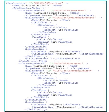
Figure 3-17. MDL Example Description of MIL-STD-1553 Data Structure
