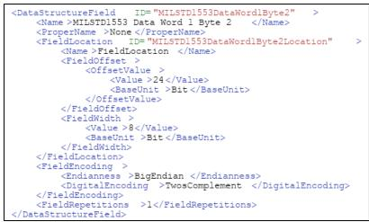
Figure 3-20. MDL Example Description of Sub-Data Word Level Field Assignments
