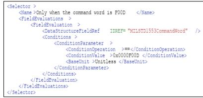
Figure 3-18. MDL Example Description of a MIL-STD-1553 Measurement Selector
