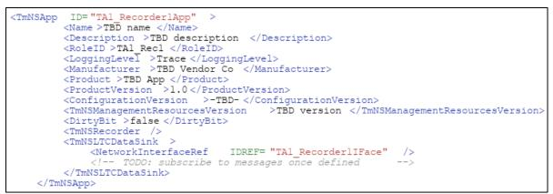
Figure 3-21. MDL Content of a TmNS Recorder Component
