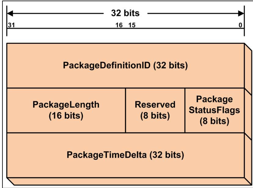
Figure 3-6. TmNS-Defined Standard Package Header
