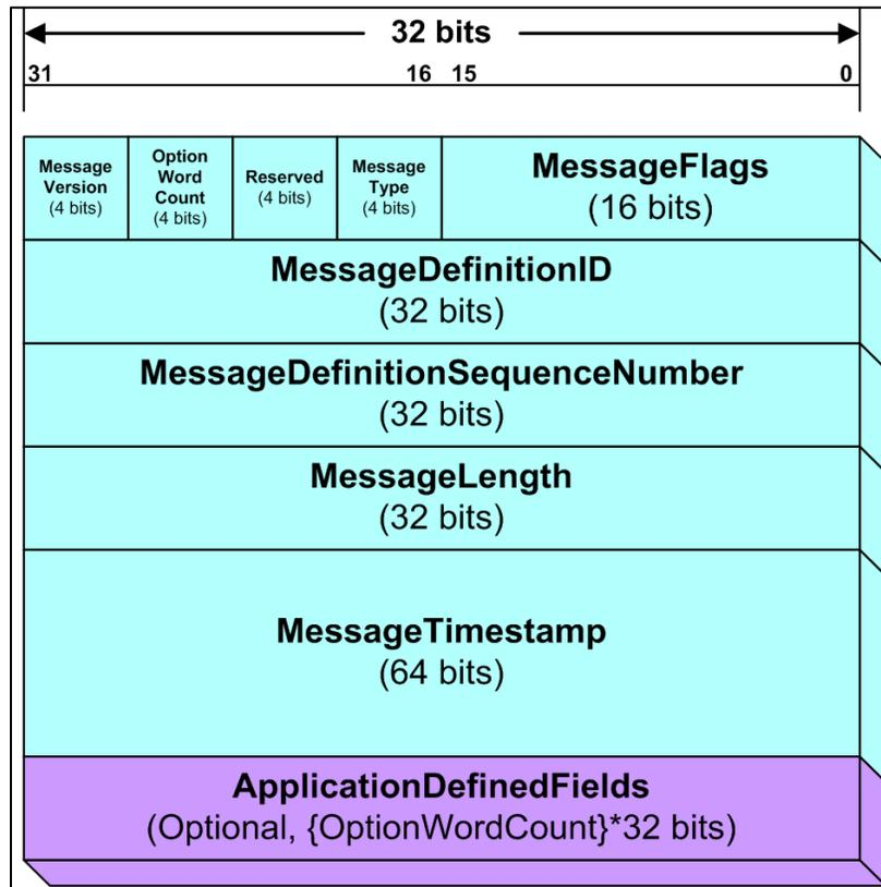
Figure 3-3. TmNS Data Message Header Structure
