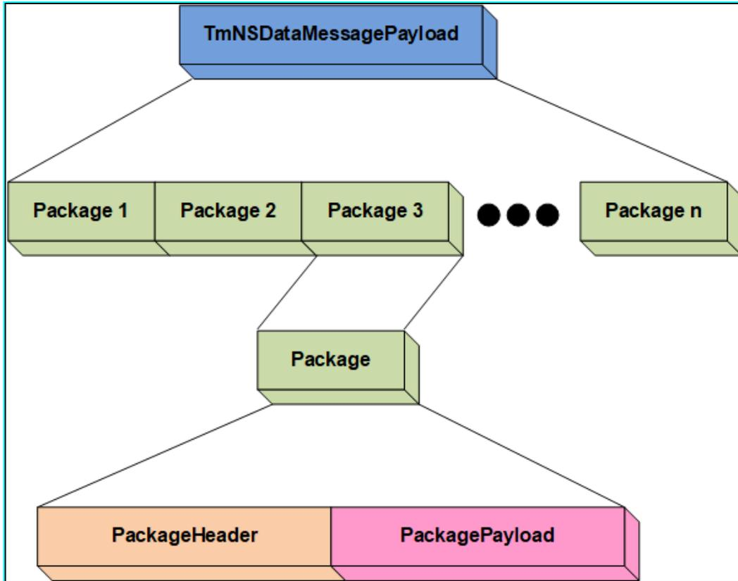
Figure 3-5. TDM Payload with Package Structure
