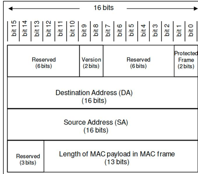
Figure 4-5. RF MAC Header Structure
