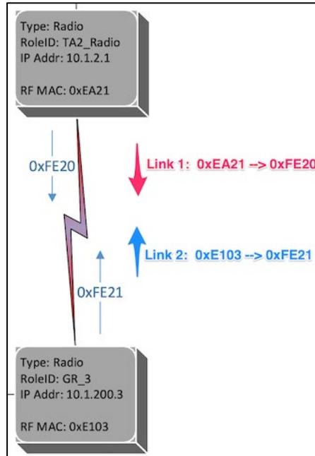
Figure 4-4. Two RF Links Required for Two-Way Communications
