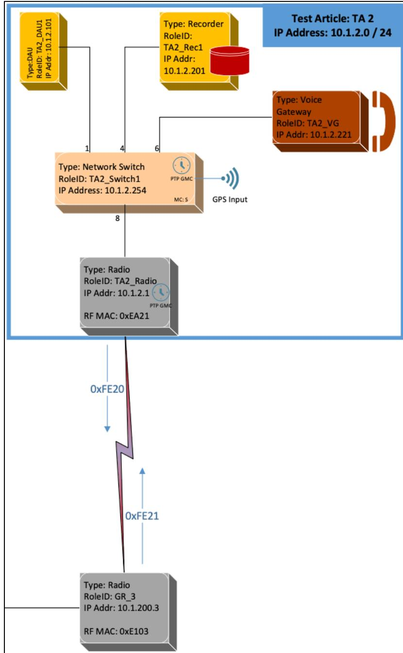
Figure 4-12. Example Topology for Static Link Scheduling
