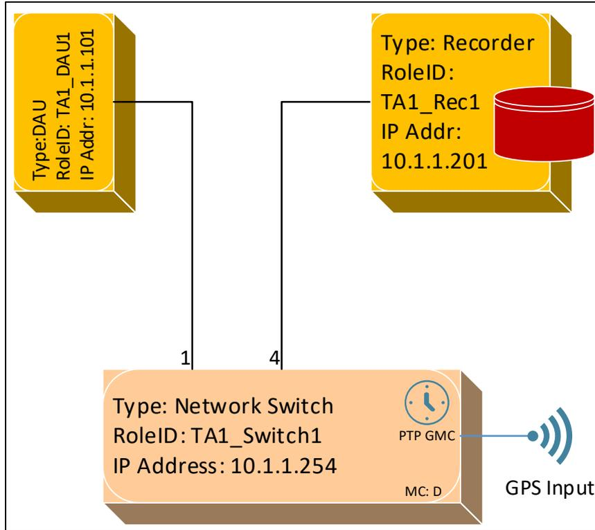
Figure 3-1. Example Components for Data Acquisition Capability on a TA
