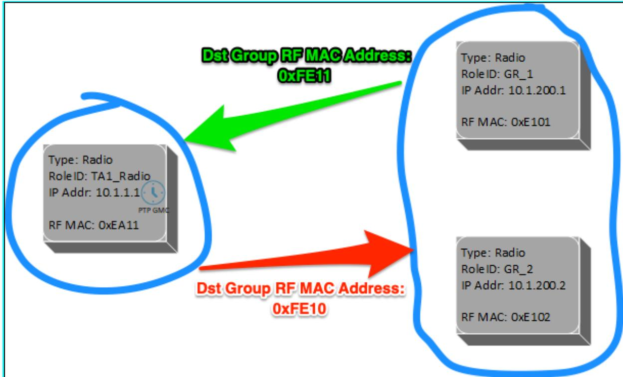
Figure 4-6. Creating RF Links for Two-Way Telemetry
