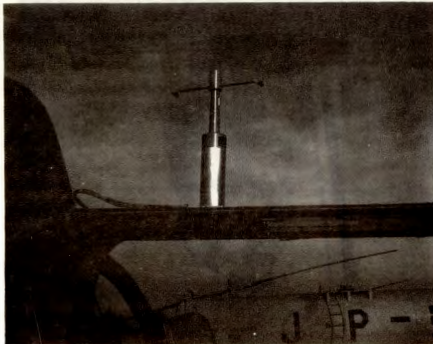
FIGURE 4 AH-1J (BuNo 157794) LORAS II MOUNTED ON CANOPY, NOV 1972
