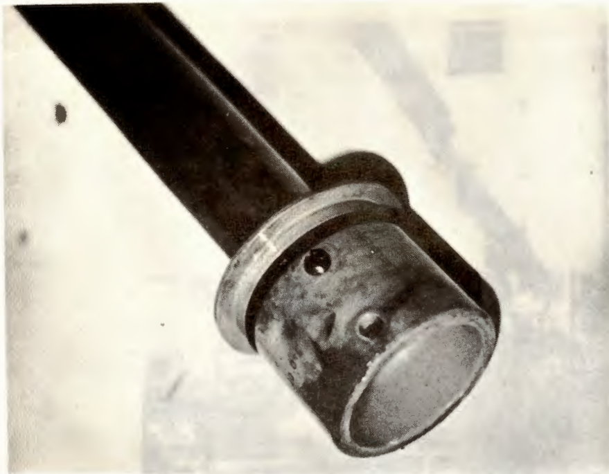
FIGURE 36 UH-1N STANDPIPE MOUNTING PLUG
