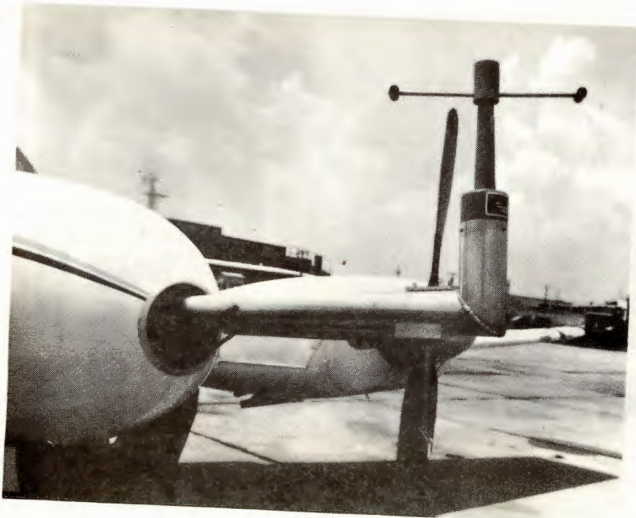
FIGURE 12 LORAS MOUNTED ON BEECH BARON NOSE BOOM
