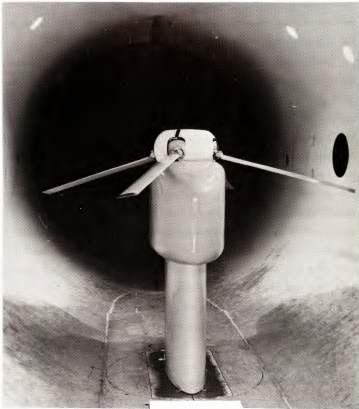
Figure 1. Helicopter rotor model in the 12-foot pressure tunnel.
