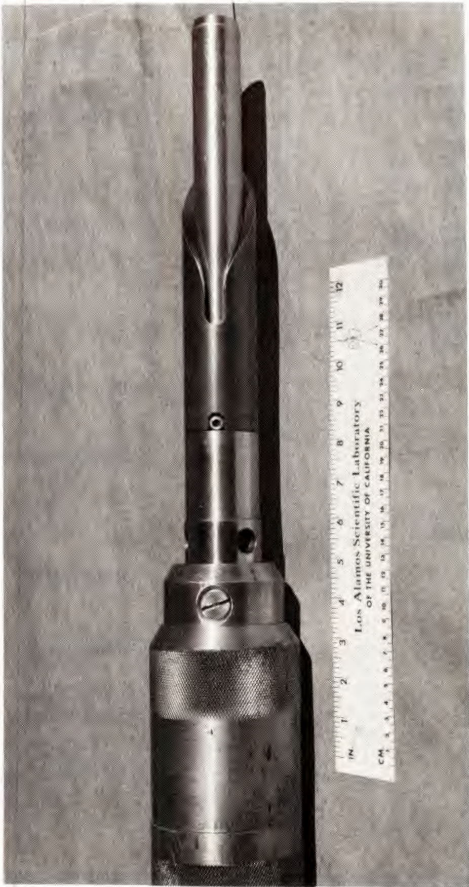
Fig. 8. Instrumentation sonde orientation mule shoe.
