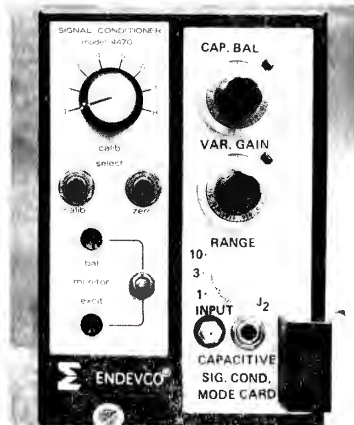
Figure 6. Signal Conditioners: Commercial Signal Conditioning Module and Custom Built Mode Card
