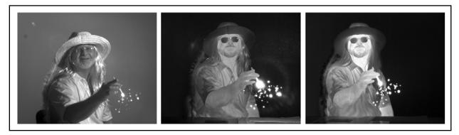
Figure 2-7. Common imagery captured in the short-, mid-, and long-wave bands.
