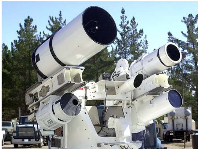
Cine-Sextant with a RC Optical lens with a 28 ½ inch outside diameter
