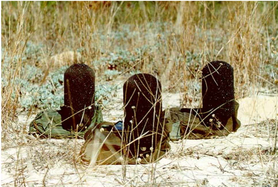
Figure 2-2. Microphones placed in direct contact with the ground surface.
