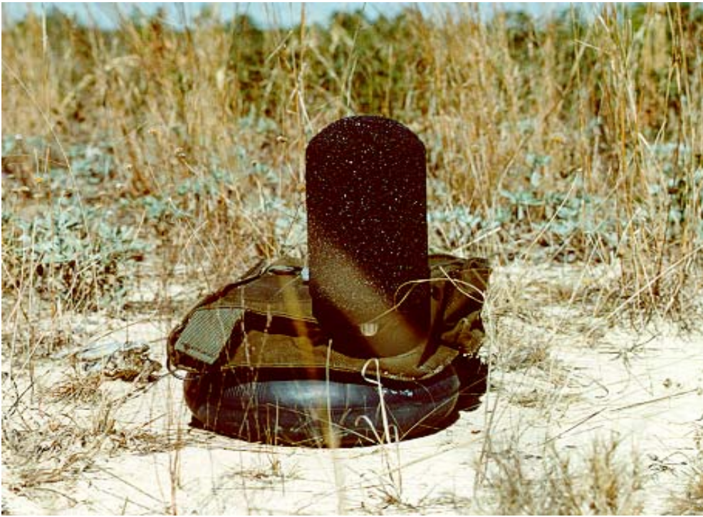
Figure 2-1. Single microphone isolated from ground vibrations.
