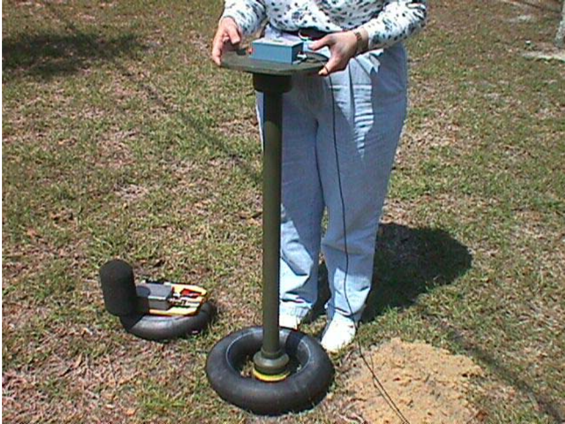
Figure 2-3. Placement of a subsurface microphone in a cavity (view #1).
