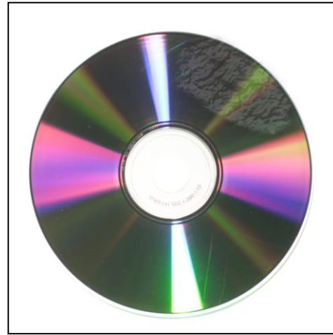
Figure 2-7. CD rot in upper right.
