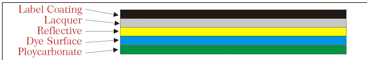
Figure 2-4. Five-layer structure of recordable discs.
