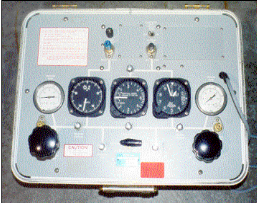
Figure 7-5. Barfield Pitot-Static Ramp Test Set
