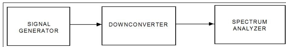
Figure 6-8. Downconverter Spurious Signal Generation
