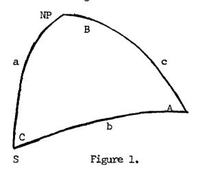
Separation angle "b" is obtained by using the cosine law to determine its cosine and hence its degrees. The degrees are then converted to distance.
