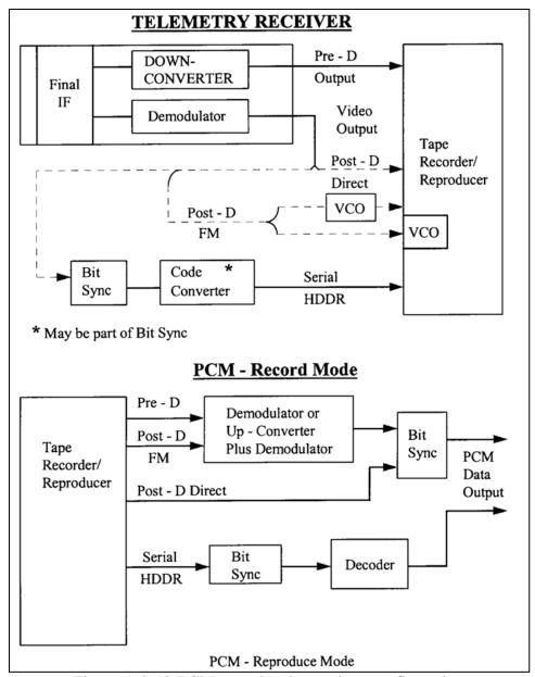
Figure A.2-12.PCM record and reproduce configuration
