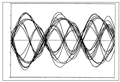
Figure A.2-5. Biφ-L at bit packing density of 15 kb/in
