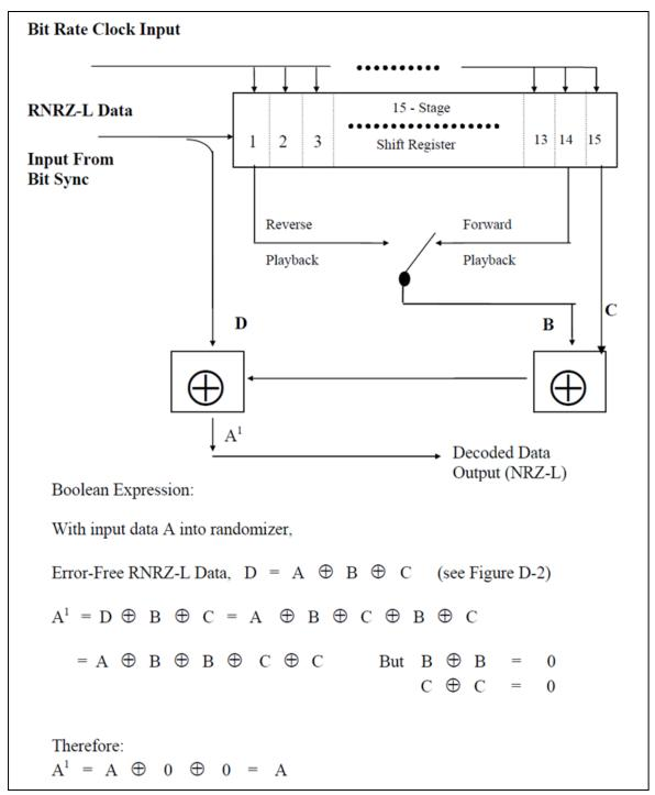
Figure A.2-3. Randomized NRZ-L decoder block diagram
