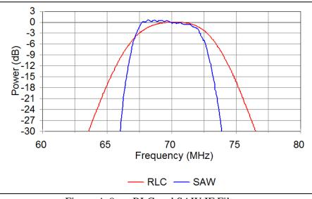
Figure A-9. RLC and SAW IF Filters
