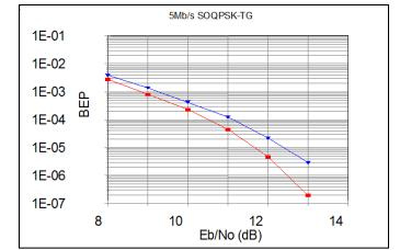
Figure A-24. BEP vs. E<sub>b</sub>/N<sub>0</sub> Performance of 5 Mbps SOQPSK-TG
