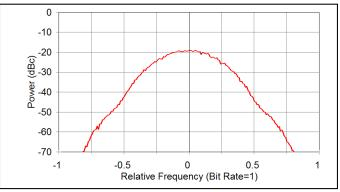
Figure A-23. SOQPSK-TG Power Spectrum (5 Mbps)
