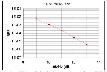
Figure A-26. BEP vs. E<sub>b</sub>/N<sub>0</sub> Performance of 5 Mbps ARTM CPM
