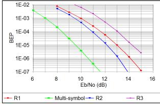
Figure A-28. BEP vs. E<sub>b</sub>/N<sub>0</sub> Performance of 5 Mbps PCM/FM with Multi-Symbol Bit Detector and Three Single Symbol Receivers/Detectors
