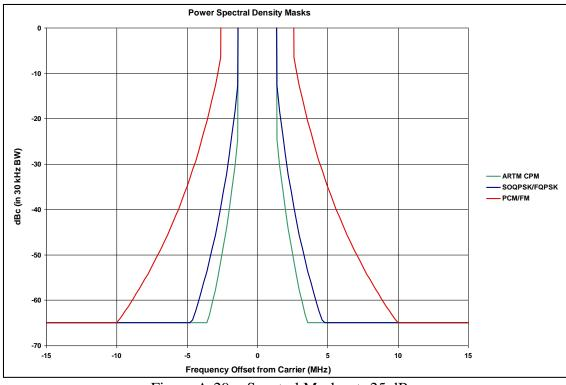
Figure A-29. Spectral Masks at -25 dBm
