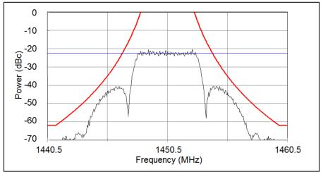
Figure A-10. Filtered 5-Mbps RNRZ PCM/FM Signal and Spectral Mask
