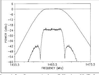
Figure A-5. Spectrum Analyzer Calibration of 0-dBc Level
