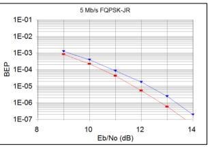
Figure A-21. FQPSK-JR BEP vs. Eb/No
