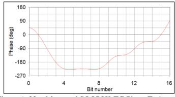
Figure A-22. Measured SOQPSK-TG Phase Trajectory
