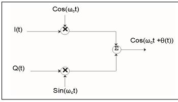
Figure A-14. OQPSK Modulator
