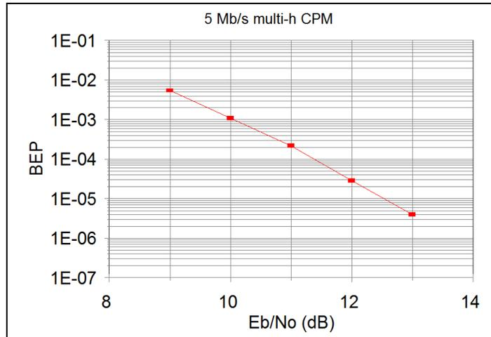
Figure A-26. BEP vs.  $E_b/N_0$  Performance of 5 Mbps ARTM CPM
