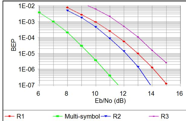
Figure A-28. BEP vs.  $E_b/N_0$  Performance of 5 Mbps PCM/FM with Multi-Symbol Bit Detector and Three Single Symbol Receivers/Detectors
